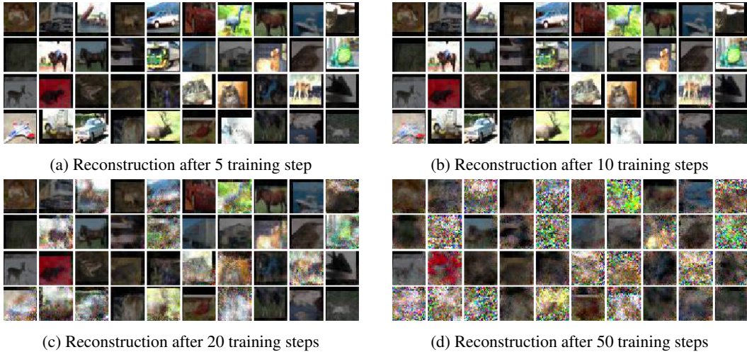
Figure 6: Our reconstruction results after several training steps with ATS, batch_size 32, and augmentations 7-4-15. We can see how the visual quality starts to decline after 10 steps and at 50 steps one can no longer reliably recover the input.
