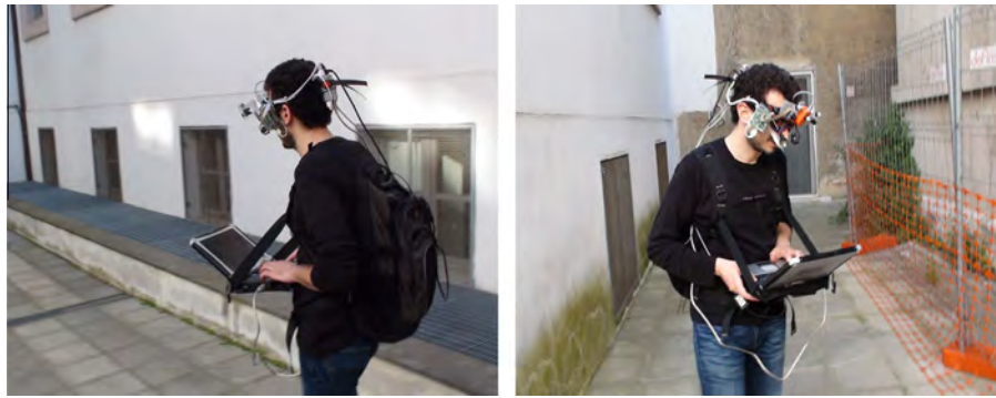
Fig. 2 The Gaze Machine (GM) worn by the subject collecting PORs in an outdoor search task.
