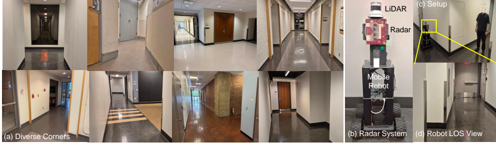
Figure 5: Experiment setup. (a) Example corners in the dataset. (b) Our radar system and robot. (c) Around-corner setup. (d) The human is occluded from the robot’s LOS view.
