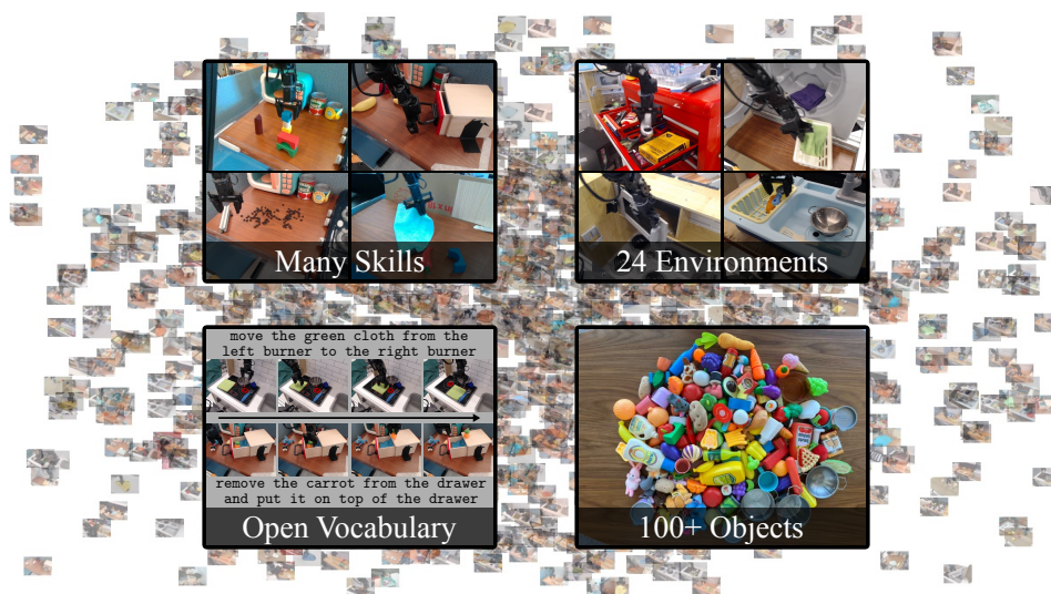
Figure 1 (BridgeData V2) We propose a large-scale robotic manipulation dataset containing 60,096 trajectories across 24 environments. The dataset includes skills such as pick-and-place, pushing, sweeping, stacking, folding, and more. Portions of the data include multiple camera views and depth data, and all of the data includes natural language labels.
