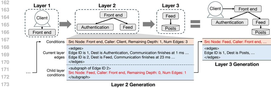
Figure 2: Overview of the recursive generation method with a simplified example. The model uses conditions generated in *Layer 1* (e.g., source node, caller, number of edges) to generate two edges in *Layer 2*, one leading to *Authentication* and the other to *Feed*. The model also generates starting conditions for the next layer, beginning from the *Feed* microservice. This recursion continues until all edges in *Layer 3* are generated.
