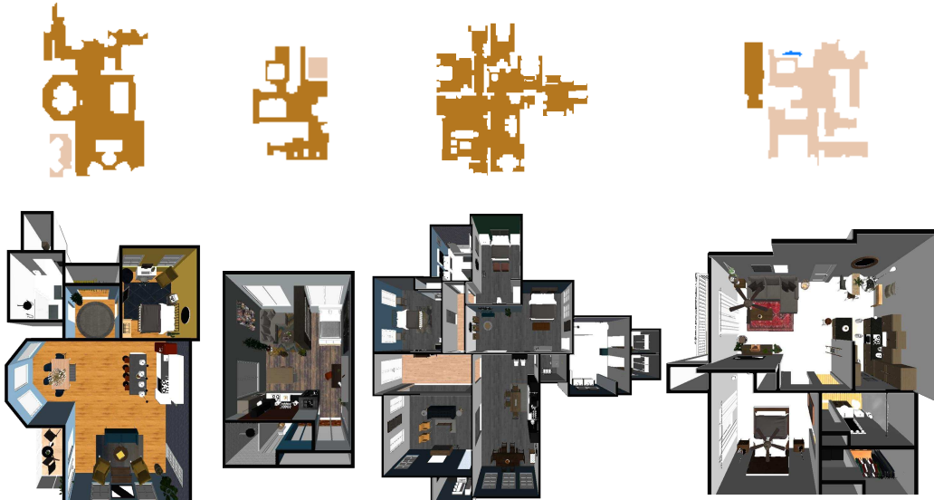
Figure 8: Visualization of the navigable geometry (top row) and top-down views of example scenes from the Habitat Synthetic Scenes Dataset (HSSD) [19]. We use the computed navigable area to efficiently generate a large number of episodes for the Open-Vocabulary Mobile Manipulation task. Object placement positions are sampled to be near navigable areas of the map, atop one of a large variety of different receptacles, such that the robot can reach them.
