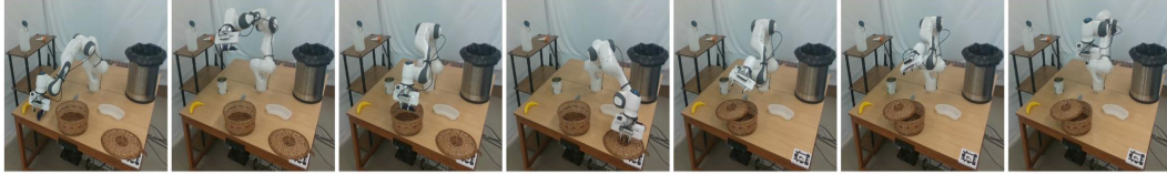
(b) The robot picks up a brinjal from the table, places it in the basket, and then covers the basket with its lid.
