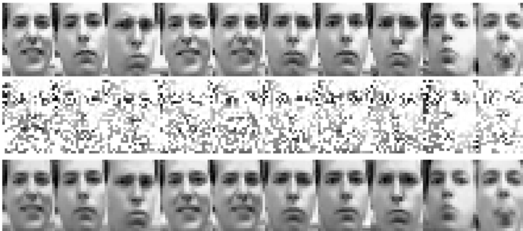
Figure 2: In the Brendan faces reconstruction task with 75% missing pixels, the top row represents the ground truth data and the bottom row showcases the reconstructions from the 20-dimensional latent distribution.
