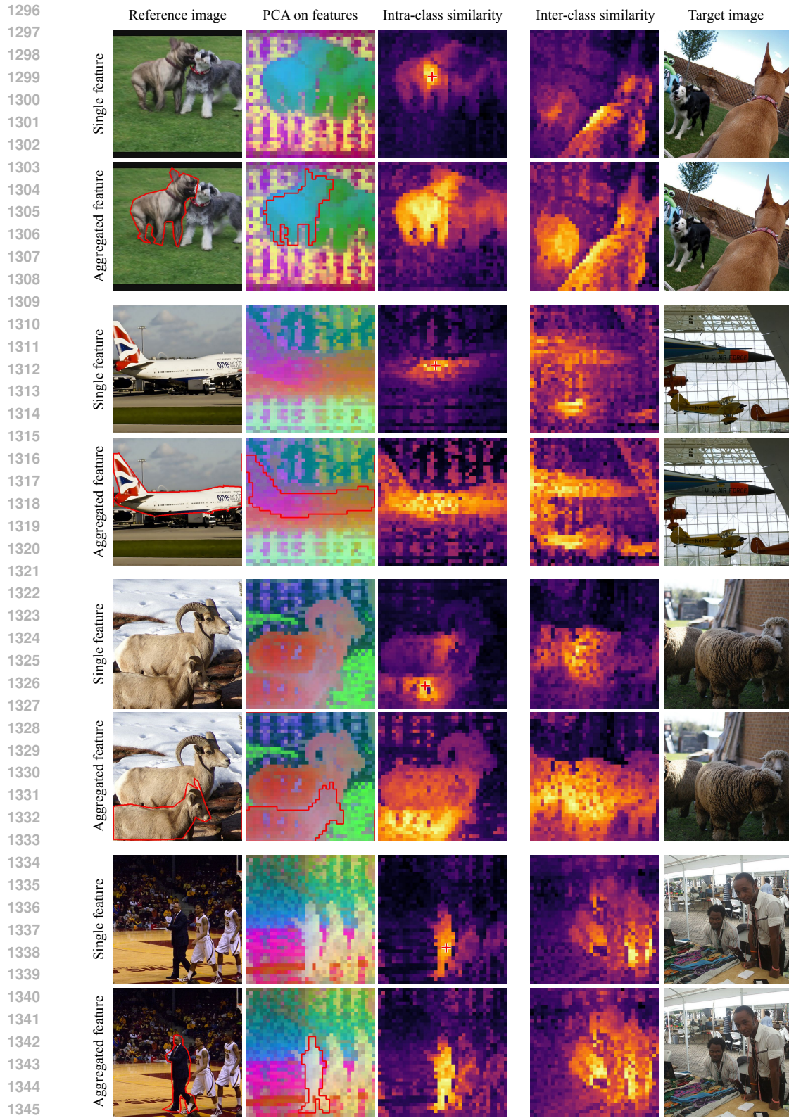
1347 Figure 17: Feature similarity — additional paired examples. For each reference-target image pair: 1348 the top row shows cosine similarity maps computed from a single DINOv2 patch feature (marked 1349 +), and the bottom row shows maps computed from the aggregated prototype (mask-area average). For each row we display intra-class (same image) and inter-class (target image) similarity. Paired examples demonstrate that aggregated prototypes yield more coherent, object-level similarity than single patch features.
