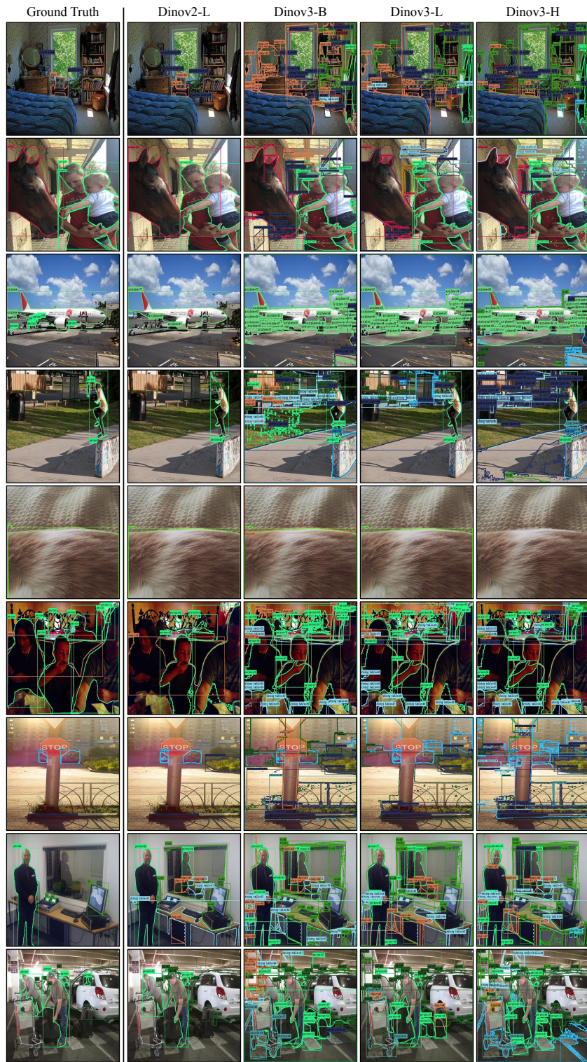
Figure 21: Output comparison across DINOv3 backbones. Comparison of training-free outputs for DINOv2-L and DINOv3-B/L/H. In DINOv3 models, higher similarity scores are often assigned to multiple proposals, and predictions show less object-focused contrast. Ground-truth masks are shown for reference.
