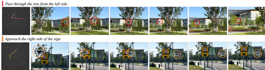
Figure 9: Visualization of real-world UAV flight demos. We deploy Pi-0-UAV, trained on UAV-Flow, on a real UAV and visualize the resulting flight trajectories alongside third-person dynamic views.
