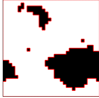
Figure 2: A typical configuration of the 2d Ising model at low temperature. Note existence of macroscopic regions of spins with \sigma_i = +1 (black) and \sigma_i = -1 (white). Domain walls are the boundary of these regions, highlighted in red.
