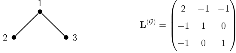
Fig. 3.3. Left: Example of an FL network \mathcal{G} with three nodes i = 1, 2, 3 that are connected via two edges with unit weight A_{1,2} = A_{1,3} = 1 . Right: Laplacian matrix \mathbf{L}^{(\mathcal{G})} \in \mathbb{R}^{3 \times 3} of \mathcal{G} .
