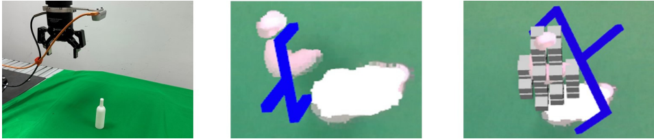
Figure 4: Comparison in real-world test. Left : a tiny bottle is right below the camera so the observation is severely self-occluded. Middle : due to the lack of complete shape, the grasp pose estimated by the baseline collides with the bottle. Right : Our method reconstructs the complete shape of the grasp region and succeeds.
