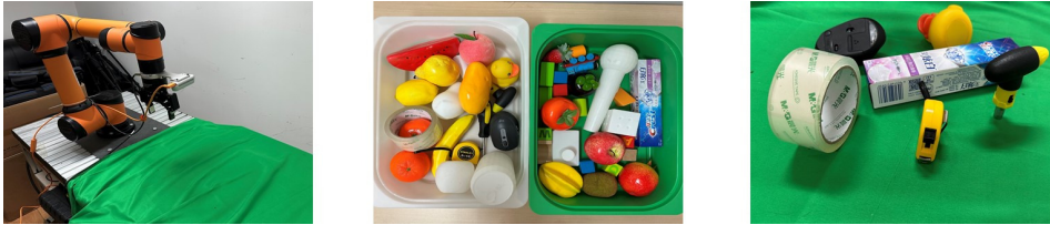
Figure 3: Settings of real-world experiments. Left : the configuration of the grasping system. Middle : objects used for grasping. Right : an example of the grasping scene.
