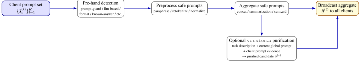
Figure 8. Server-side defense and aggregation. The server filters suspicious prompt updates, preprocesses the remaining prompts, aggregates them, and optionally performs task-anchored purification before broadcasting the next-round global prompt.
