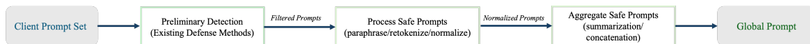
Figure 5. Server-side defense and aggregation. The server filters suspicious prompt updates, preprocesses the remaining prompts, aggregates them, and optionally performs task-anchored purification before broadcasting the next-round global prompt.
