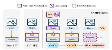
Figure 4: **Overview of different training algorithms** for multimodal policy internalization. The solid purple outlines indicate the parts where the next-token prediction loss is computed. On the right, we illustrate the proposed three-stage training strategy, TriMPI, which enables direct policy knowledge injection through the VM-CPT stage and policy-grounded reinforcement learning through PolicyRollout. The PolicyRollout algorithm is detailed in §4.3 and illustrated in Figure 5.
