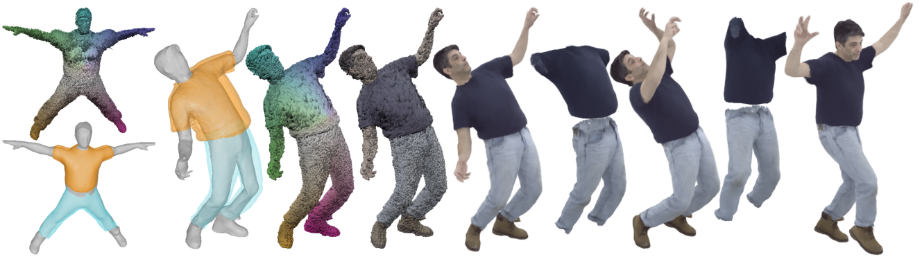
Figure 1. Given a multi-view video input, D3GA is trained to create light, drivable, photorealistic 3D human avatars. These avatars are constructed as a composition of 3D Gaussians encapsulated within tetrahedral cages. The Gaussians undergo transformation and stretching influenced by these cages, are colored using an MLP, and are rasterized into splats. By representing the drivable human as a collection of 3D Gaussian layers, we gain the ability to decompose and manipulate the avatar as needed.
