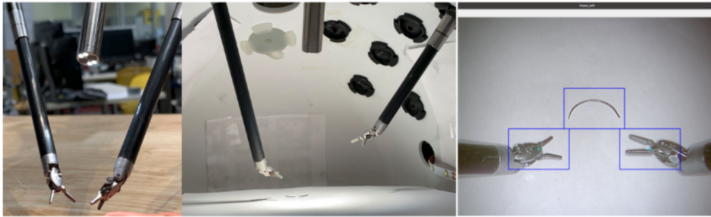
Figure 3: (Left) close up view of the dVRK arms, camera, and the integrated light source, (middle) experimental setup, with a box as a platform and piece of paper as a background, (right) workspace view from the camera perspective; blue squares indicate the general starting locations of the grippers and the suture needle
