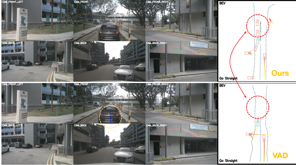
Figure 3: Visualization. This figure compares LAW in the perception-based setting with VAD (Jiang et al., 2023). On the right side of this figure, we display the results of ego trajectory prediction, agent motion prediction, and map construction in BEV. As indicated by the red circles , our method captures more crucial scene information, which VAD overlooks. Consequently, VAD predicts a forward trajectory that results in a rear-end collision, as highlighted by the yellow circles .
