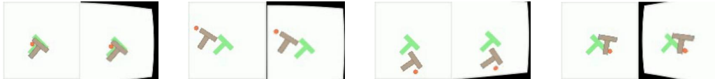
Figure 5: Visualization examples of noisy Push-T dataset. Each subfigure shows the effect of condition noise, where the left image is the original image observations and the right image is the corresponding version with added camera distortion.
