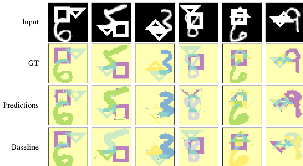
Figure 13: Weakly supervised semantic segmentation results on the MNIST2Shape dataset. The baseline creates accurate object masks, albeit with wrongly predicted labels due to its random matching process. Our proposed approach leveraging Rotating Features, on the other hand, falls short in creating accurate semantic segmentations.
