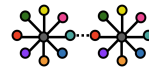
Figure 2: Double star with random bridge. The prior knowledge graph G consists of two disjoint star graphs on the left and right. The ground-truth graph G^* adds a single, hidden “bridge” edge between random leaves on the left and right. Any algorithm must query \Omega(n) leaves on average to find this bottleneck edge.
