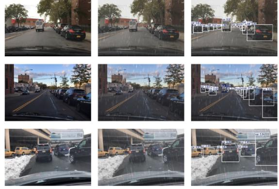
**Figure 2.** Qualitative evaluation of YOLOv8++ over synthetic rain generated and augmented data. Column 1: Original images, Column 2: Rain-augmented images, and Column 3: Bounding boxes generated by YOLOv8++ model
