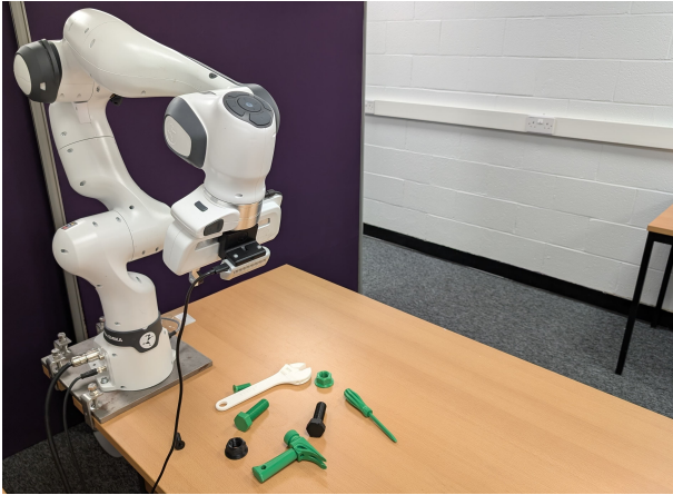
Figure 3: Our experimental setup: the Franka Emika Research 3 is equipped with a Intel RealSense D435i RGB-D camera on its gripper. It collects pictures from several points of view by moving over a hemispherical trajectory.
