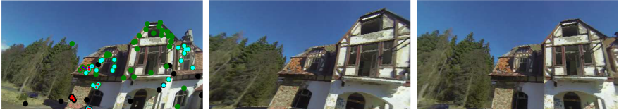
Fig. 1. Removing RS and radial distortion simultaneously using our minimal absolute pose solver. The original image (left) with tentative correspondences (black) the inliers captured by P4Pfr+R6P [4] (blue) and subsequent local optimization (red) compared to inliers captured by the proposed R7Pfr (cyan) and subsequent local optimization (green). The correction using R7Pfr without local optimization (right) is better than by P4Pfr+R6P with local optimization (middle). (Color figure online)
