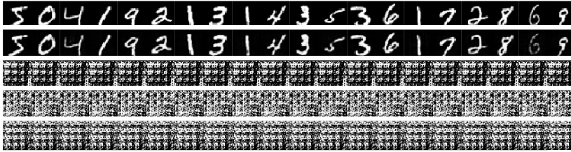
Figure 1: Reconstruction results of FSHA against the guest’s data in the first row. The following rows are attack results against the original SplitNN and our solution ( \epsilon = 0.1, 1.0, 4.0 ), respectively.
