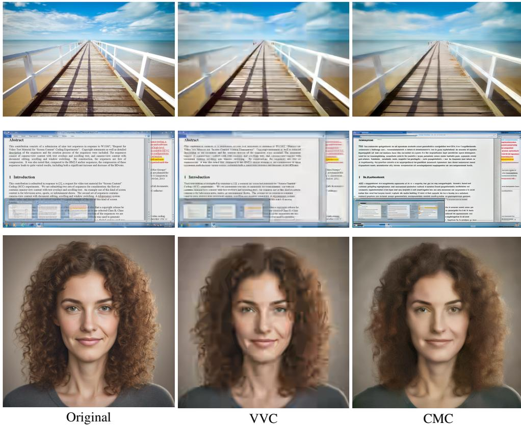
Figure A17: Success and failure cases for CMC. Left is the original image, the middle is compressed by VVC, right is compressed by CMC (GPT-4o+RealVis). NSI/SCI/AIGI cases are shown from up to bottom. The bitrate is fixed at about 0.024bppps. We found CMC is more successful than the advanced VVC, in the upper NSI and bottom AIGI; however, for the middle SCI, both of them cannot draw the words on the website, but at least CMC is not blurry. Zoom in for details.
