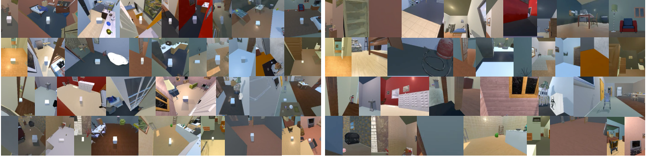
Figure 11. Random embodiments in the AI2-THOR simulator. Right column shows the egocentric view from the main camera and the left column shows a third-person view of the agent –white boxes indicate the robot colliders for visualization purposes only.
