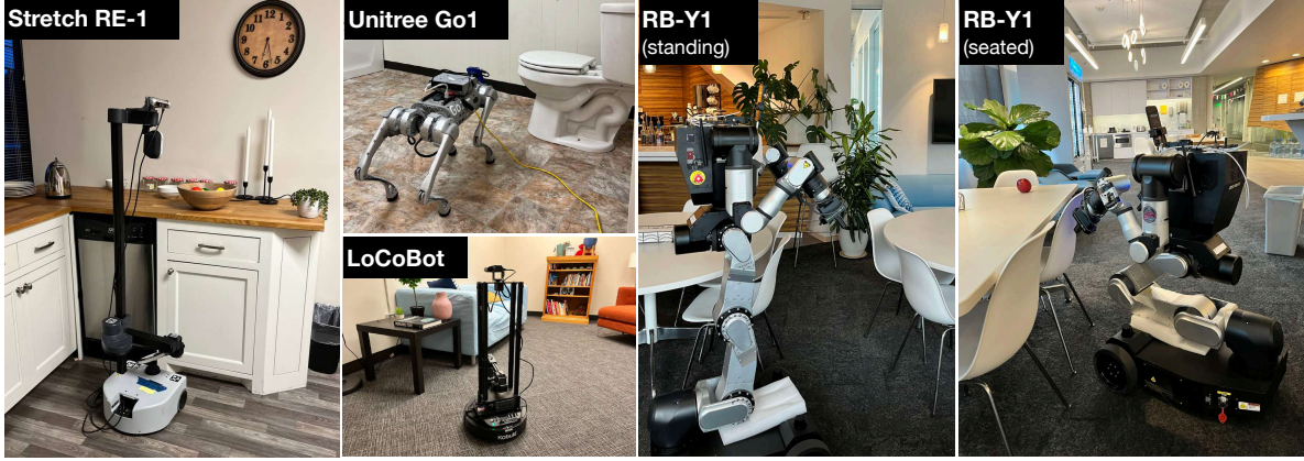
Figure 7. Robot platforms. We use 3 different platforms, including Stretch RE-1, LoCoBot, and Unitree GO1 for our real-world evaluations.
