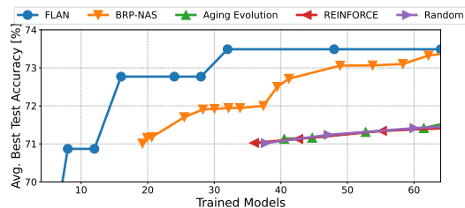
Figure 10: FLAN with the iterative sampling search algorithm (BRP-NAS) outperforms other popular search methodologies on NASBench-201 CIFAR100.
