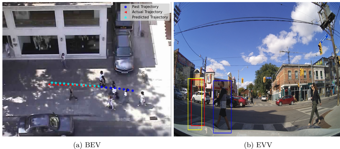
Figure 6: Sample images of the deterministic prediction from BEV datasets (a.) (ETH and UCY) and EVV dataset (b.) (PIE). The Red and Yellow bounding box indicates the ground-truth and predicted final position respectively and the Blue bounding box indicates the start position.
