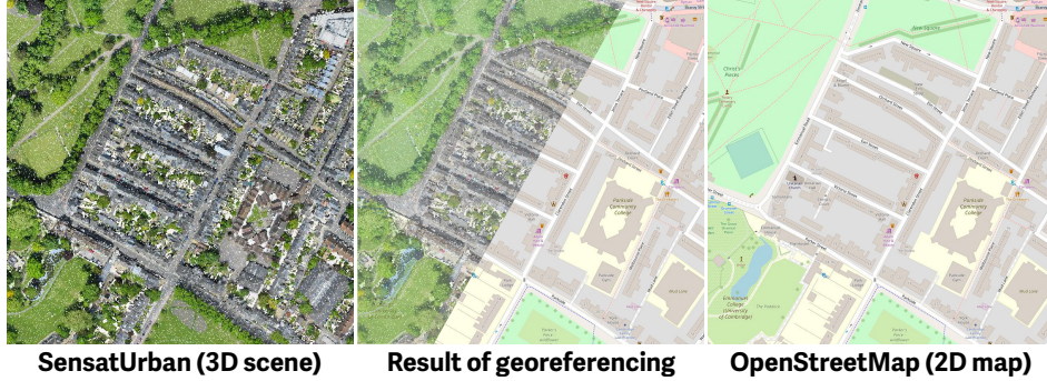
Figure 3: Georeferencing of 3D environment and 2D map.
