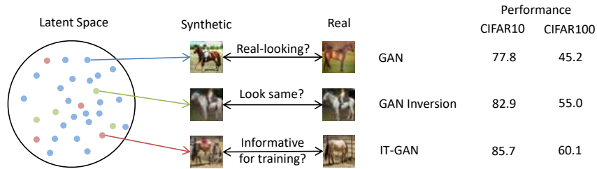
Figure 1: Different objectives and performances of traditional GAN, GAN inversion (1) and our IT-GAN. BigGAN (5) architecture is used in all three methods. We learn latent vectors in the latent space of a pre-trained GAN that correspond to informative training samples. We show that our IT-GAN achieves better performance than traditional GAN and GAN inversion on CIFAR10/100 when being used as the training data generator.
