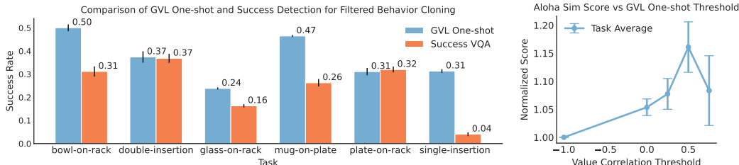
Figure 6: Success-Filtered Imitation Learning on ALOHA Simulation Tasks. Left: Using GVL-SD for success-filtered BC substantially outperforms SuccessVQA. Right: GVL-SD is not sensitive to the VOC threshold for improving imitation learning.
