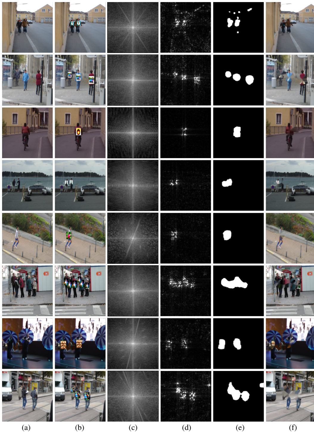
Figure 14: (a) A benign image. (b) A Naturalistic patch applied to the image. (c) The frequency domain. (d) The cut image. (e) The patch mask after denoising. (f) The attacked image inpainted based on the patch mask.
