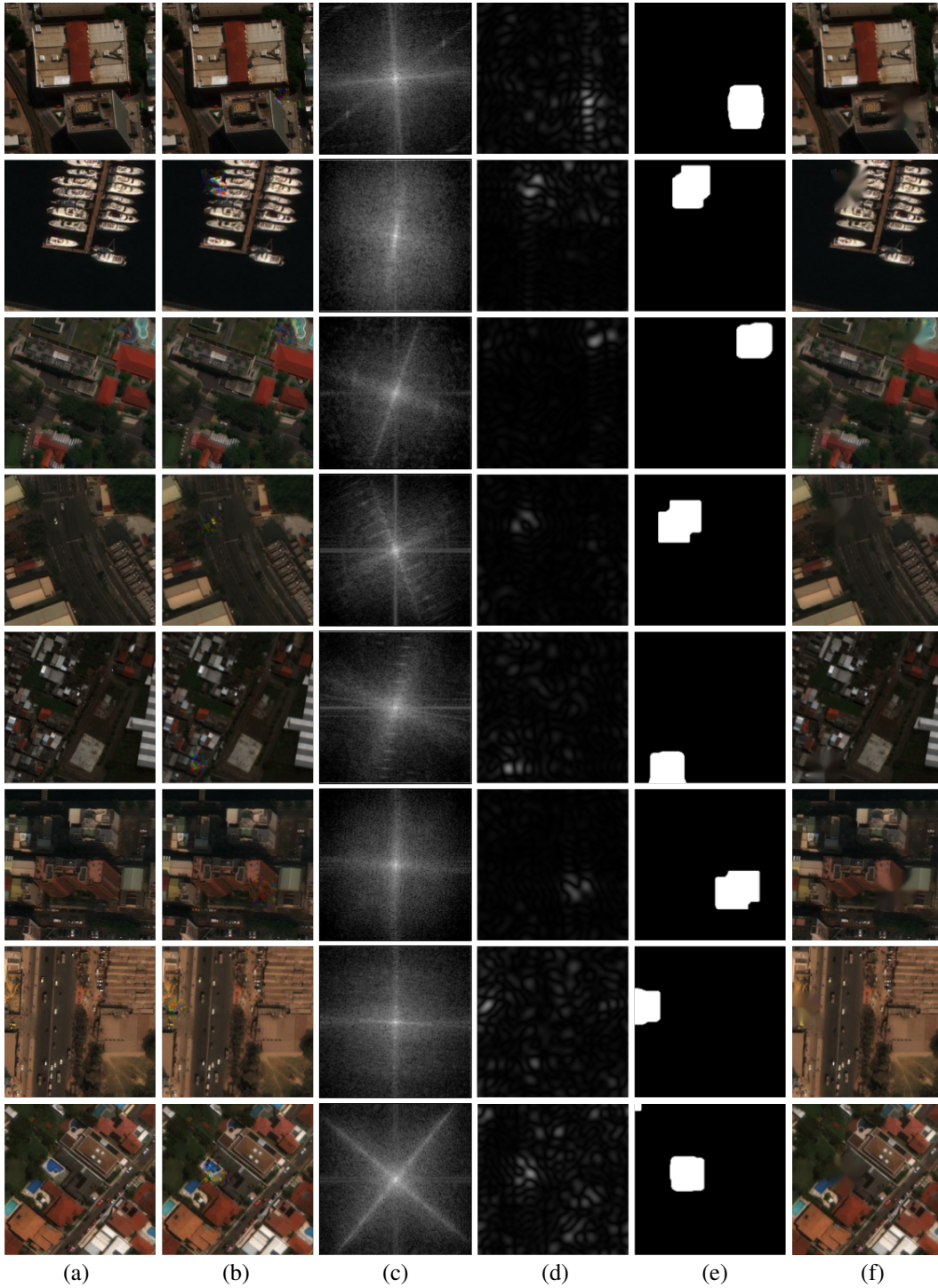
Figure 13: (a) A benign image. (b) A PGD patch applied to the image. (c) The frequency domain. (d) The cut image. (e) The patch mask after denoising. (f) The attacked image inpainted based on the patch mask.
