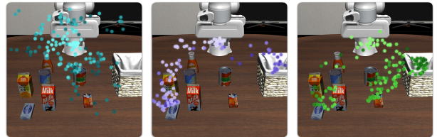
Fig. 10: Comparison of exploration behaviors on the task, “pick up the butter and put it in the basket” for RLPD (left), DSRL (center), and TMRL (right). While RLPD expands coverage via action noise and DSRL relies on actions from the conditional distribution, TMRL leverages action sequences from smoothed contexts, resulting in broadened, yet coherent exploration.
