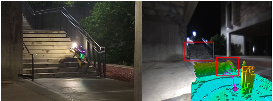
Figure 6: Scene used to tell the robot to “Run upstairs” and “Go to the second floor”. The second sentence fails due to the code trying to “count floors”
