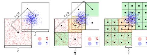
Figure 3: Recursive partitioning of  $\mathbf{X}$  and  $\mathbf{Y}$  for 2D data. Far-field interactions are colored green while near-field interactions are colored orange and  $\delta$  denotes the euclidean distance between the centers.
