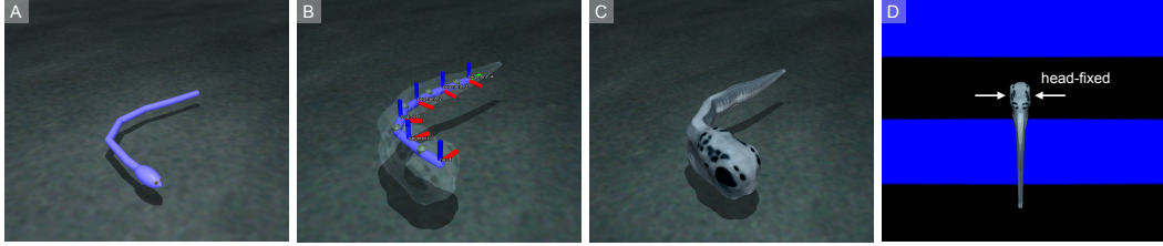
Figure 1: Simulation of the zebrafish agent in a physics-based virtual environment. A) The 6-link embodiment geometry [1] in a environment with dynamic fluid forces. B) The agent controls the torque exerted by motors at each joint (5 DoF) to swim and navigate its environment. C) A custom cosmetic skin to mimic the appearance of larval zebrafish. D) A virtual environment matching the experimental parameters of the open loop protocol Mu et al. [2]. The root joint located at the head is fixed during training.
