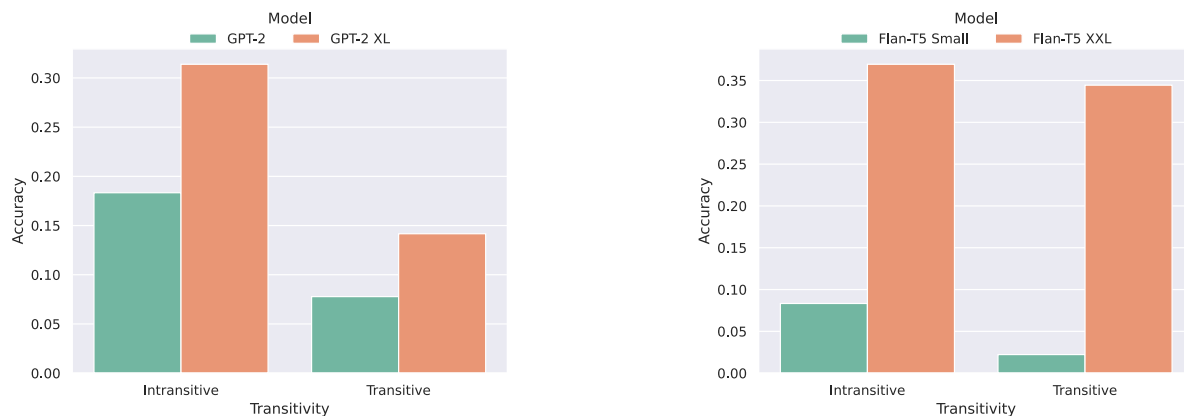
Figure 1: Accuracy for transitive and intransitive verbs on smaller and larger language models. Random baseline accuracy is 0.292. The smaller models perform worse than random (due to nonsequitur outputs) and the larger ones do slightly better than random. Larger models clearly vastly outperform smaller ones.
