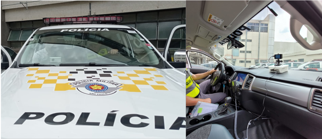
Figure 3: Deployment in Police patrol vehicles. The Sentinel device is powered by the car’s battery and it is kept on whenever the vehicle’s engine is also on.
