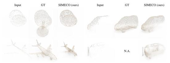
Figure 13: **Failure cases.** Top: ambiguous partial scans leave the network unsure how to complete the shape. Bottom: poor input quality disrupts the transform restoration module and yields misalignment.
