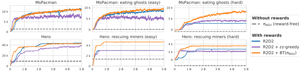
Figure 5: Scores in Atari games with modified reward functions. We train a single task-agnostic policy per environment, and leverage it to solve three different tasks: the standard game reward, a task with sparse rewards (easy), and a variant of the same task with deceptive rewards (hard).
