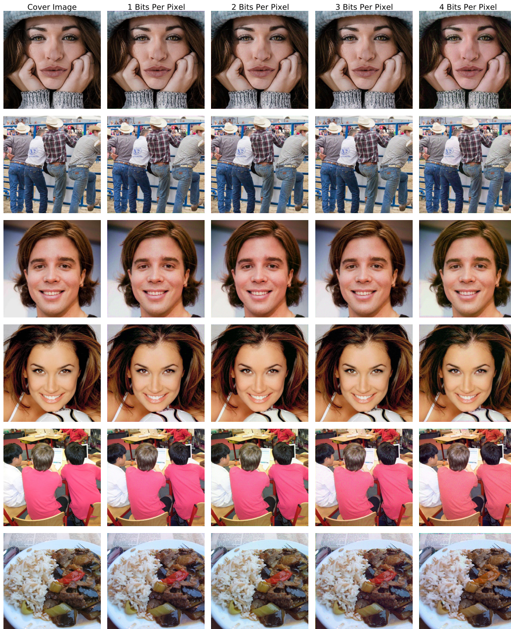
Figure 8: Cover images with corresponding steganographic images under different payloads. The first 2 images are from Div2k, the following 2 are from CelebA, and the last 2 are from MS-COCO.
