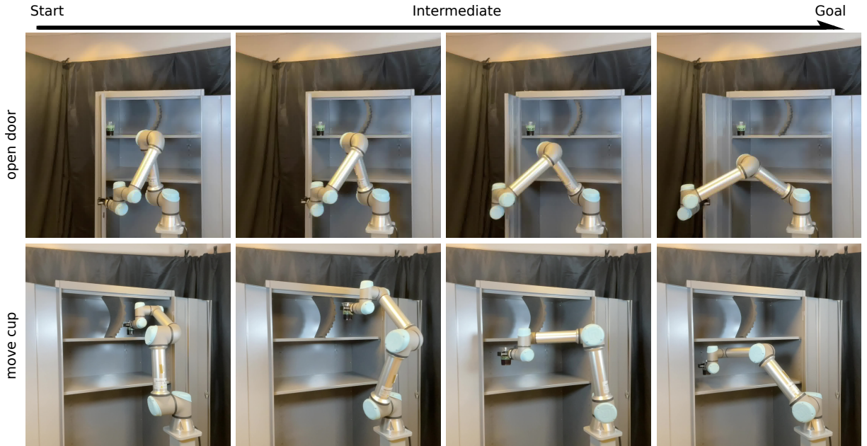
Fig. 3: Two different real-world manipulator cases: the first row shows the door opening task, whereas the second shows the manipulator moving an object from the cabinet’s top shelf to the lower shelf by crossing two relatively thin obstacles.
