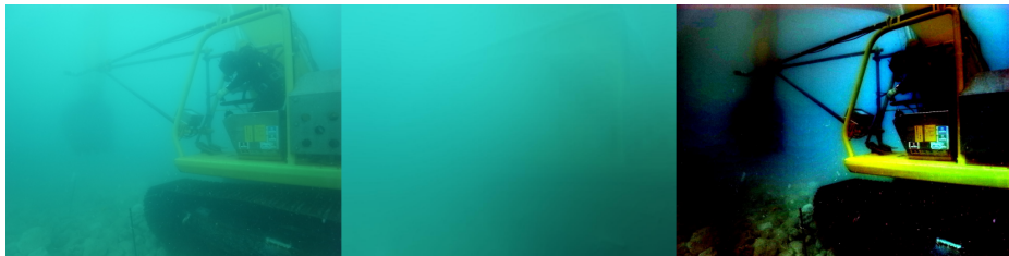
Fig. 2. Input image (1st column), the top Laplacian pyramid component of the image (2nd column), and result of subtraction of the top component from the original input (3rd column). We experimentally found that the top Laplacian pyramid component of a degraded underwater image dominates noise signal, and just removing the component tends to extract original signal. The 3rd column is multiplied by ten for visualization.
