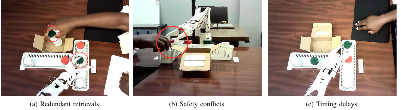
Fig. 4: Recurring failure modes observed in Human-Agent collaboration: (a) redundant retrievals due to opaque robot intent, (b) safety conflicts from simultaneous access to shared shelf space, and (c) timing delays from uncertainty about the next robot’s subtask
