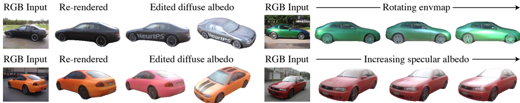
Figure 8: Our SG method allows for artistic manipulation of appearance, such as novel view synthesis, material editing (both diffuse and specular components), and relighting, thanks to our effective disentanglement.
