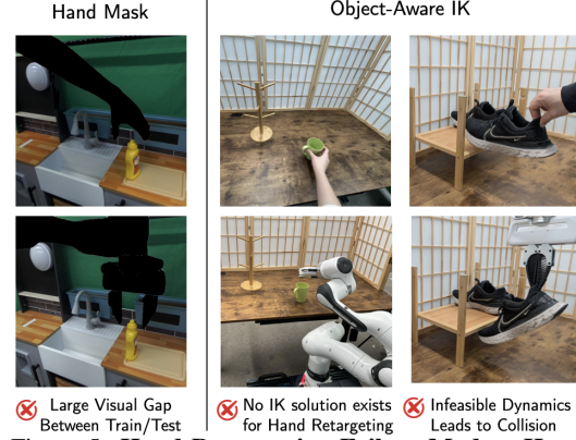
Figure 5: Hand Re-targeting Failure Modes: Hand Mask fails due to a significant visual domain gap between human and robots, even when the motions are physically feasible for the robot. Object-Aware IK fails under execution mismatch, as certain human hand motions are kinematically or dynamically infeasible.
