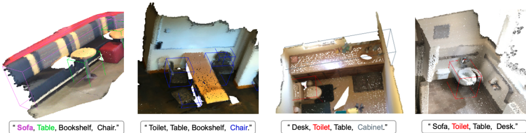
Figure 4: Qualitative results for open-vocabulary 3D object detection results. For each scene, the detection prompt is shown under the input point cloud. The colors of bounding boxes correspond to the classes in the prompts.
