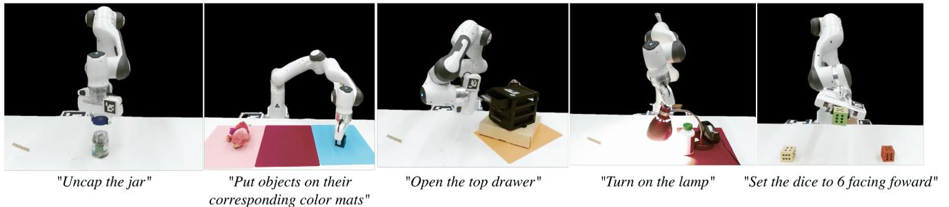
Fig. 3: Manipulate-Anything is an open-vocabulary autonomous robot demonstration generation system. We show zero-shot demonstrations for 12 tasks in simulation 5 tasks in the real world.
