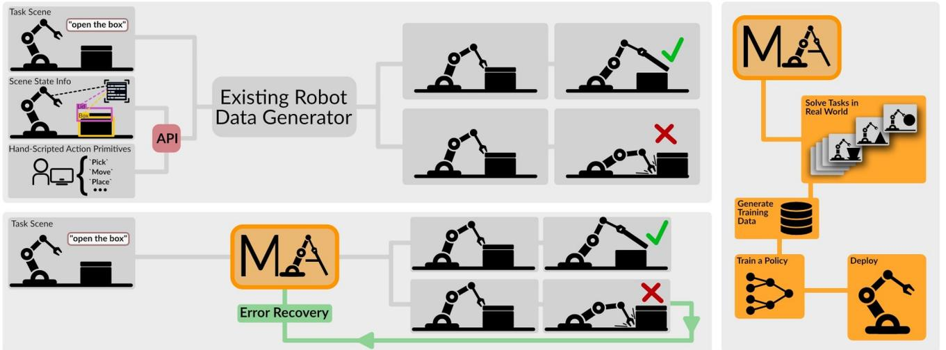
Fig. 1: Manipulate-Anything is an automated method for robot manipulation in real world environments. Unlike prior methods, it doesn’t require privileged state information, hand-designed skills, or limited to manipulating a fixed number of object instances. It can guide a robot to accomplish a diverse set of unseen tasks, manipulating diverse objects. Furthermore, the generated data enables training behavior cloning policies that outperform training with human demonstrations.
