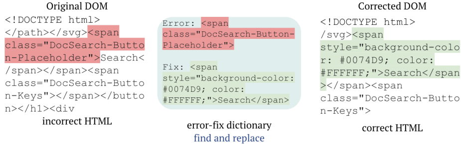
Figure 6: Example DOM correction process for one individual violation. This process was repeated for all violations in the dataset.
